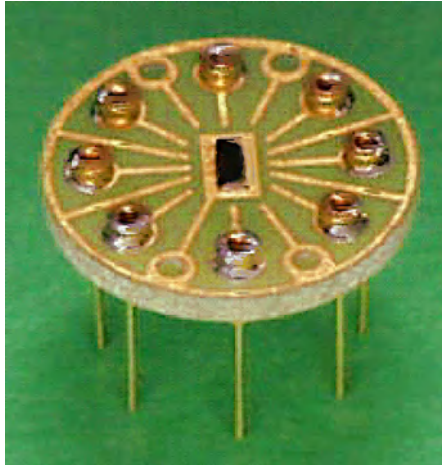
Figure 3.2: The EUROMET holder printed circuit board where the QHE sample is bonded.
