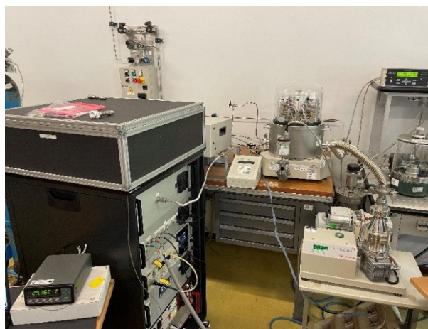
Figure 7: System installed at INRiM. The pressure balance can be seen on the table behind the TOP.
