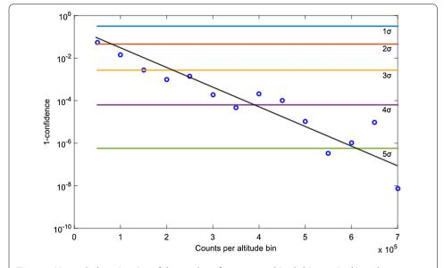
Figure 7 Monte Carlo estimation of the number of counts per altitude bin required in order to confirm (or refute) Eq. (2) to a specified confidence. Horizontal lines indicate increasing 'sigmas' of confidence, descending from  $1\sigma$  to  $5\sigma$ . The simulated Monte Carlo data are represented by circles, and the sloped line is an exponential fit to the generated data.
