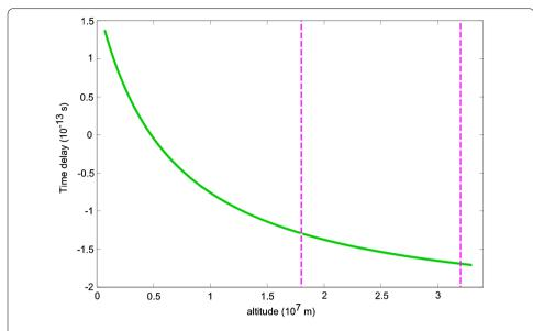
Figure 2 The total time delay between the fibre clocks, as a function of height, for a fixed fibre length and fibre refractive index. The dashed lines mark lowest and highest altitudes at which measurements could be performed (see feasibility analysis). In this region the time delay is dominated by the Shapiro delay. The choice of fibre length and refractive index is discussed in Section 3. The altitudes and orbital parameters are discussed in Section 5.
