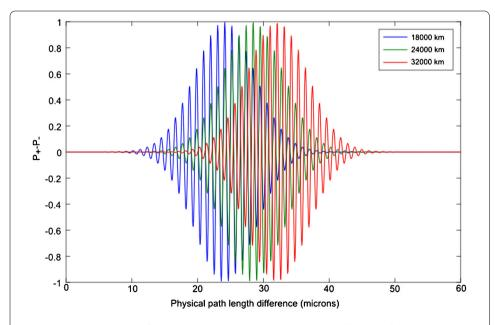
Figure 3 The expected interferometer signal vs. physical path length difference of the two interferometer arms, with the parameters as described in the text, at three different heights of the satellite. The signal was calculated by numerically evaluating Eq. (2) with a frequency-dependent refractive index as described in [18]. Increasing satellite height has the effect of increasing the mean physical path length difference, thus shifting the signal rightward.
