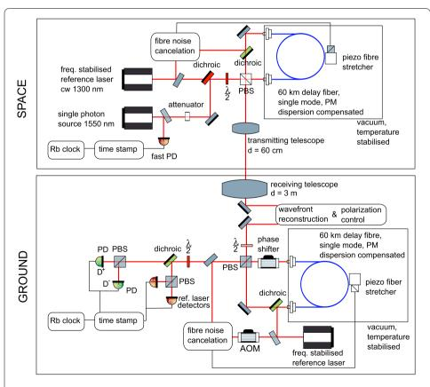
**Figure 4 Full schematic of the payload optical system.** Key: PD: photodetector; PM: polarisation-maintaining; PBS: polarising beamsplitter; AOM: acousto-optic modulator. The setup is designed to minimise the effects of other degrees of freedom besides the Shapiro delay that may introduce distinguishability at the output of the interferometer.
