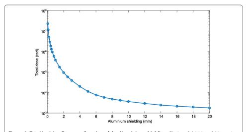
**Figure 9 Total Ionizing Dose as a function of the Aluminium shielding.** Choice of shielding thickness is a compromise between continued performance of the optical fibres and payload weight.
