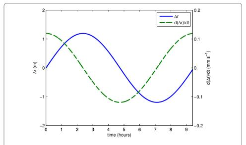
**Figure 5 Path length difference and velocity difference vs. time, due to motion of the satellite.** The solid blue line shows the free-space path length difference, and the dashed green line shows the rate of change of this difference. This is compensated for in post-processing, rather than in-flight.
