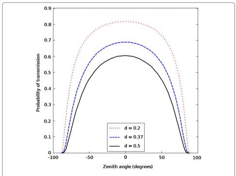
Figure 6 Probability of a photon to be transmitted through the atmosphere with respect to zenith angle,  $\theta$ , and various optical depths,  $\mathbf{d}$ . Increasing the optical depth,  $\mathbf{d}$ , has the effect of reducing the peak probability of transmission. An optical depth,  $\mathbf{d}$ , of 0.5 corresponds to high levels of pollution. Further calculations assume  $\mathbf{d} = 0.37$ , giving an atmospheric transmission probability of 0.69 at zenith.
