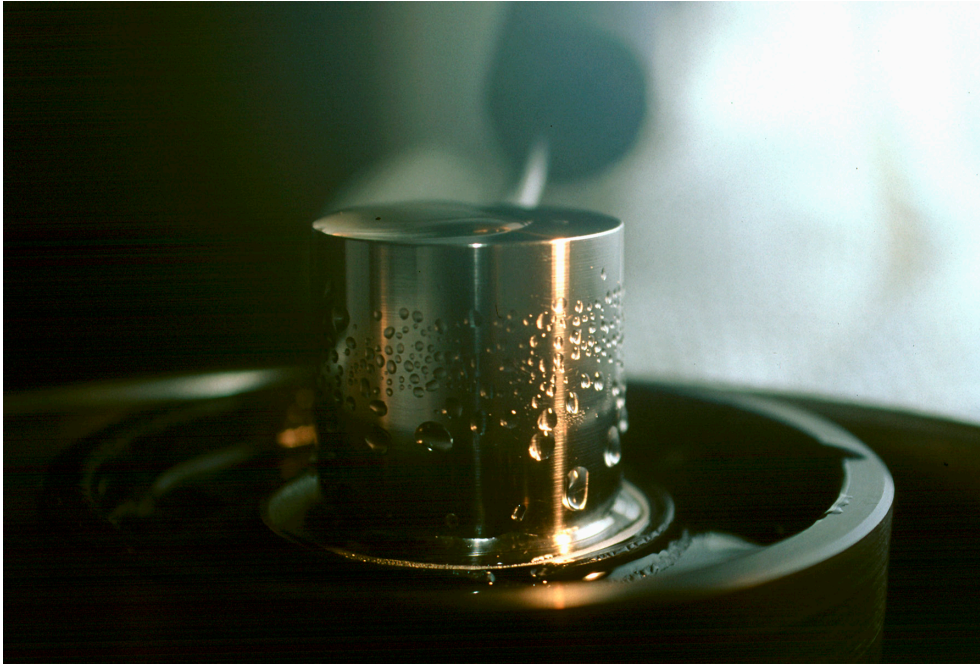
Fig. 4. – The Italian mass standard, the Pt-Ir prototype n. 62, during cleaning-washing at the INRiM.
