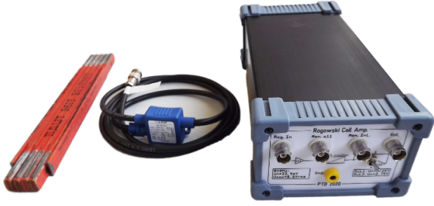
Fig. 7: Rogowski coils with the corresponding electronic integrator.
