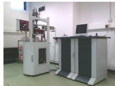
Figure 13: Primary Hardness Standard Machine at INRiM
