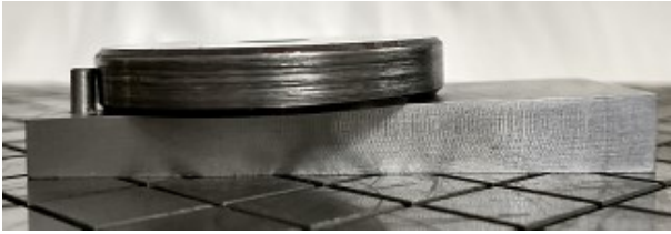
Figure 3: Arrangement of the hardness block on the angled block
