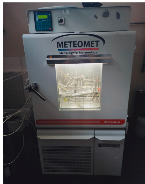
Figure 1. Climatic chamber Kambic MeteoCal KK-105 in operation at INRiM and used to test RS92 and RS41 under various temperature and humidity conditions and ambient pressure. The chamber simultaneously and independently controls temperature (range -40\text{ }^{\circ}\text{C} < T < 180\text{ }^{\circ}\text{C} ) and relative humidity (range 10\% < RH < 98\% in the temperature range 10\text{ }^{\circ}\text{C} < T < 95\text{ }^{\circ}\text{C} ).
