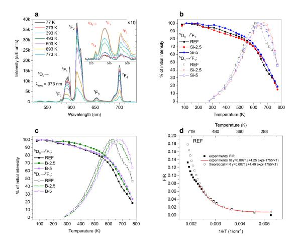
**Fig. 2**. (a) Thermally dependent  $Eu^{3+}$  emission spectra of REF glass excited at 375 nm. (b,c) Luminescence intensity of the transitions from  ${}^{5}D_{0}$  and  ${}^{5}D_{1}$  levels to  ${}^{7}F_{1}$  level for REF, Si-2.5, Si-5 samples (b) and REF, B-2.5, B-5 samples (c) as a function of temperature. (d) Theoretical and experimental FIR for the REF glass, taken as an example.
