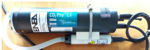
Fig. 4 - CO 2 -Pro CV probe on bench.
