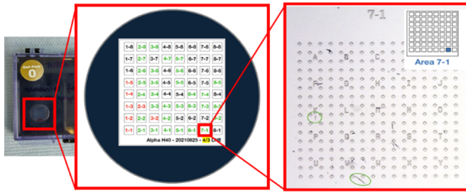
Figure 2. (left) Photography of one of the three samples used for the study. (center) Schematic view of the different numbered zone on a substrate. (right) Optical microscope view of a numbered zones (here zone 7-1) on a marked silicon substrate (9 mm × 9 mm) where are deposited nanowires. Distance between two crosses is 15 µm.
