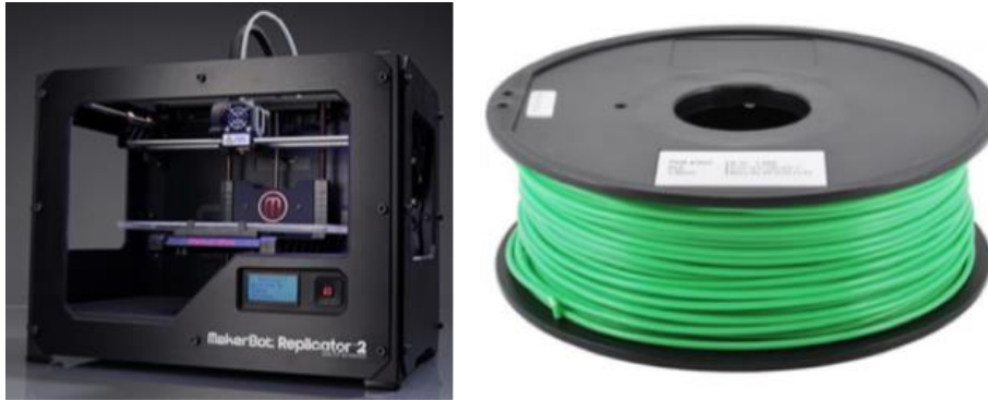
Figure 2: The 3-D printer (left) and a PLA filament bundle (right) used for the realization of the samples.
