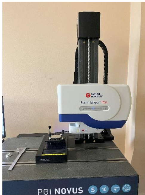
FIGURE 5 - TAYLOR HOBSON FORM TALYSURF PGI NOVUS S10
