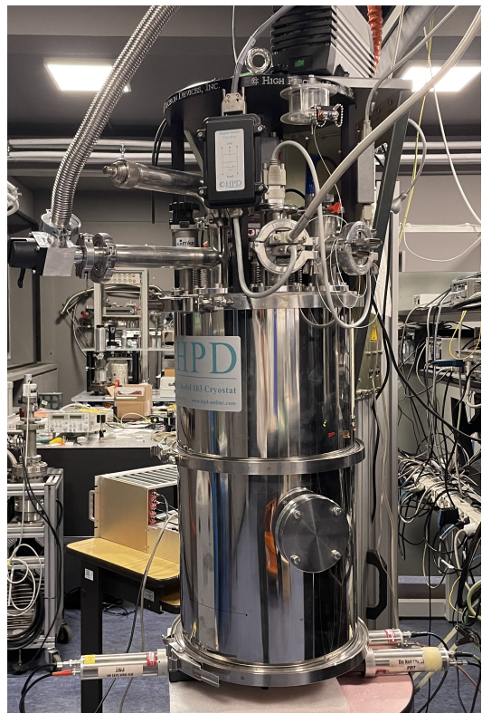
FIG. 4. The experimental setup during the cosmic ray coincidence test. The three sabers, placed side by side, are directly below the ADR.
