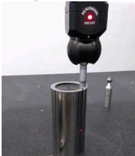
Fig. 6. Measurement of the cylinder square.
