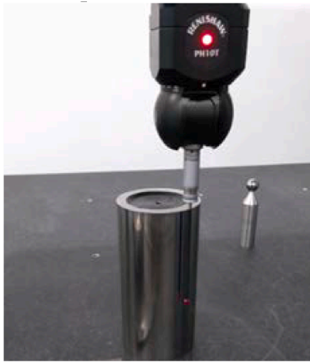
Fig. 6. Measurement of the cylinder square.
