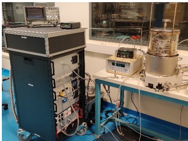
Figure 8: System installed at LNE and LNE-CNAM. The pressure balance (PG-7607 with automatic weight changing system) can be seen to the right of the TOP.
