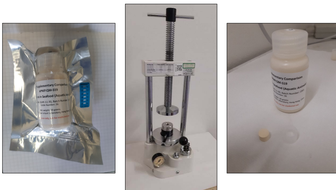
Figure 1: The comparison material (left), the manual hydraulic press used to prepare samples (center) and a pressed cylindrical tablet sample (right).
