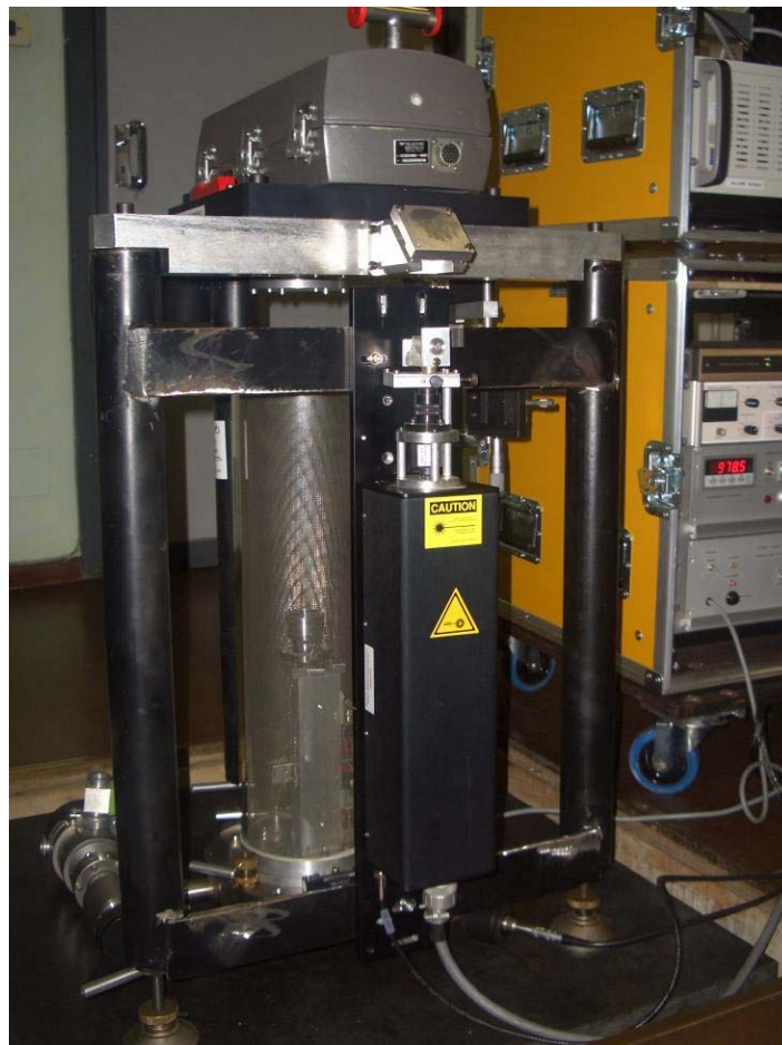
Figure 1. Picture of the absolute gravimeter IMGC-02
