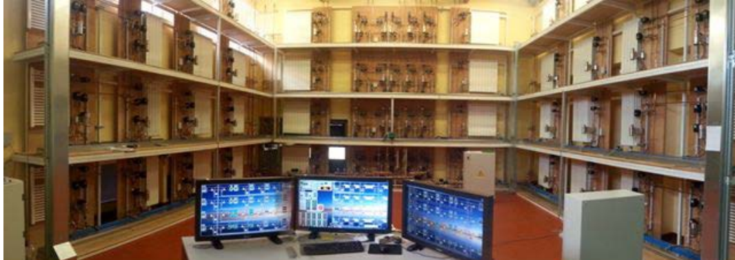
Fig. 3. The INRIM centralized heating system mock-up.
