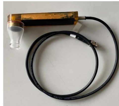
Fig. 3. INRIM transducer comprising an SU103 S/N 101, Sonic Concepts transducer with stand-off cone, which was filled with deionized, degassed water, and fitted with a Mylar acoustic window for measurements.
